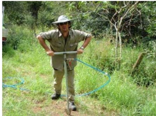
Left: Quik Spray Unit – remote-control, retractable reels, 600 L tank and fire fighter pump. Right: Aqua Spear – planting with pressurised water.
